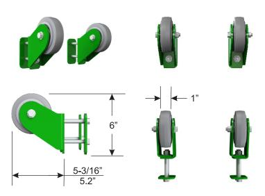
The V6WK wheel kit is designed to bolt directly to the V6 bottom frame on either the left of right. 4" diameter medical grade casters with 1" tread width make it easy to move the unit over most surfaces. With the V6 front and back outriggers locked in the upright position, this wheel kit allows you to simply tilt the V6 onto the wheels and move it just about anywhere. Assembly is required.
